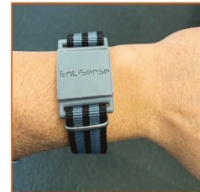
Wearable sweat sensor worn on lower arm
